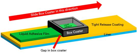
Figure 2 BYK Box Coater usage illustration
